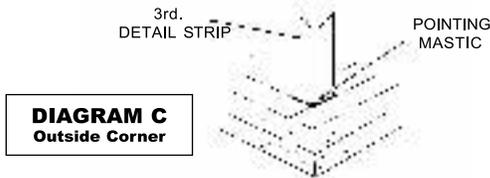
To the top terminations, apply POINTING MASTIC at least 1/8" (3.18 mm) thick and 1" (25.4 mm) wide. As an option, TERMINATION BAR may be used to mechanically fasten the membrane.
