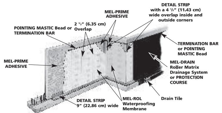
**Inspect and Repair ...** A thorough inspection should be made before covering and all necessary repairs made immediately. Tears and inadequate overlaps should be covered with MEL-ROL ... slit fishmouths and patch. Seal edges of all patches with POINTING MASTIC. Where applicable, horizontal applications can be flood-tested for 24 hours. All leaks should be marked and repaired when membrane dries.
